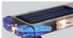
Optional solar panel compensates for parasitic draw.
